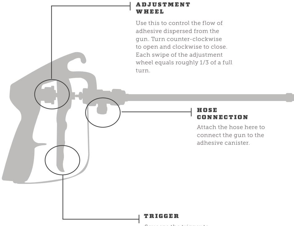
The UNO-FOAM™ Gun is the exclusive applicator for UNO-FOAM™ QD3000 48 Squares Insulation Adhesive. For optimal performance and a clean bead every time, UNO-FOAM™ should only be applied with the UNO-FOAM™ gun. *Not compatible with web spray contact adhesives, primers, or fleeceback adhesives.*
