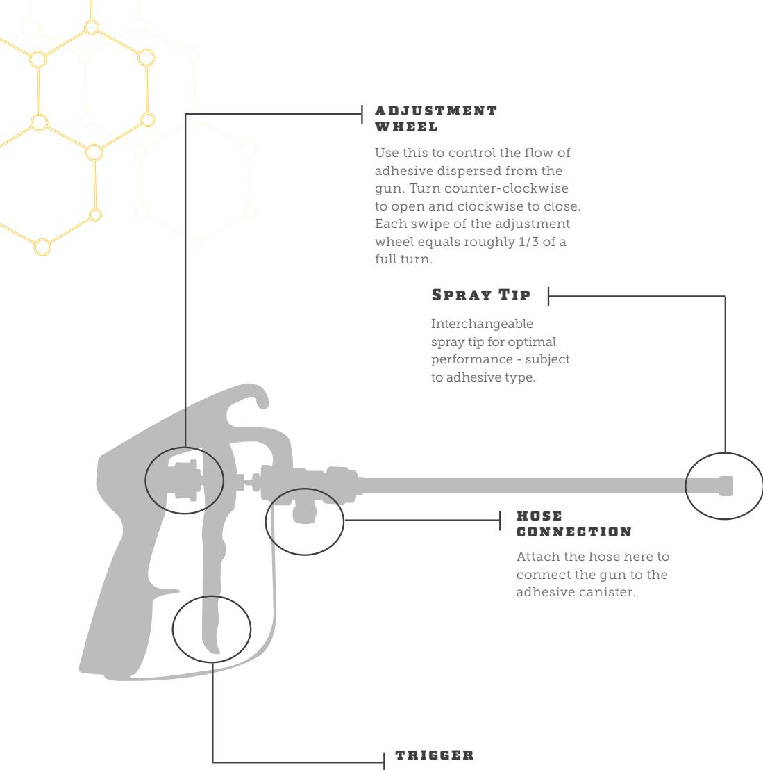
The Field Gun is designed for applying adhesive across large field areas. The long wand eliminates the need for users to bend/kneel down while applying adhesive, removing strain on the back and knees and allowing for a comfortable experience during adhesive application.
