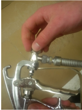
1. Unscrew tip retainer
