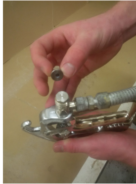
2. Lay spray tip on top
