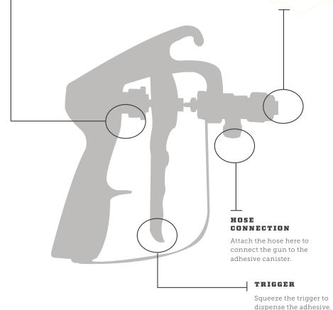
The Detail Gun is designed for applying adhesive onto smaller areas like parapets or upstands, where close attention to adhesive coat weight is critical prior to the bonding of waterproofing membrane or self-adhesive VCL's.
