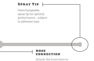
Attach the hose here to connect the gun to the adhesive canister.
